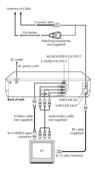
■ To connect to a TV with S-VIDEO/AUDIO input connectors . . .
